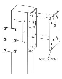
Figure 9 Aligning Adapter Plate with Mounting Plate
